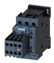
power contactor, AC-3 17 A, 7.5 kW / 400 V 2 NO + 2 NC, 24 V AC, 50 Hz, 3-pole, Size S0 screw terminal Removable auxiliary switch
