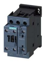
power contactor, AC-3 17 A, 7.5 kW / 400 V 1 NO + 1 NC, 230 V AC, 50 Hz, 3-pole, Size S0 screw terminal
