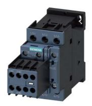
power contactor, AC-3 17 A, 7.5 kW / 400 V 2 NO + 2 NC, 230 V AC, 50 Hz, 3-pole, Size S0 screw terminal Removable auxiliary switch
