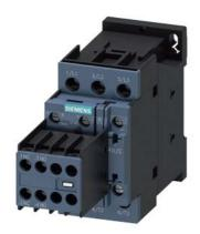
power contactor, AC-3 17 A, 7.5 kW / 400 V 2 NO + 2 NC, 220 V AC, 50 Hz, 240 V, 60 Hz, 3-pole, Size S0, screw terminal Removable auxiliary switch
