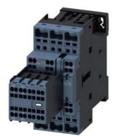
power contactor, AC-3 17 A, 7.5 kW / 400 V 2 NO + 2 NC, 110 V AC, 50 Hz, 3-pole, Size S0 Spring-type terminal Removable auxiliary switch
