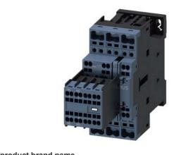
power contactor, AC-3 17 A, 7.5 kW / 400 V 2 NO + 2 NC, 230 V AC, 50 Hz, 3-pole, Size S0 Spring-type terminal Removable auxiliary switch
