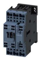
power contactor, AC-3 17 A, 7.5 kW / 400 V 1 NO + 1 NC, 220 V AC, 50 Hz, 240 V, 60 Hz, 3-pole, Size S0, Spring-type terminal
